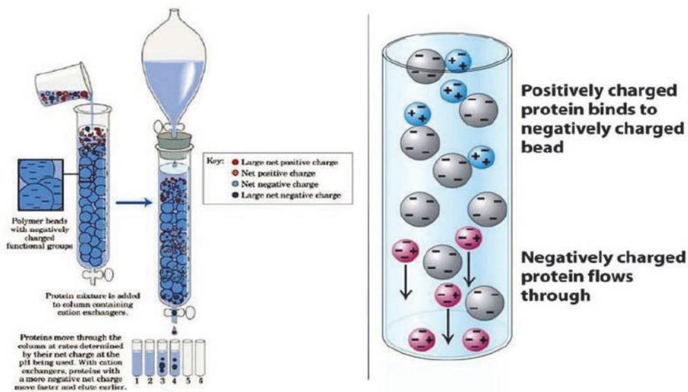
**Fig.37. Ion Exchange Chromatography**
