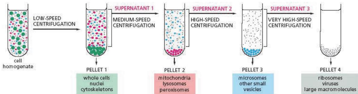
**Fig.26.2. Differential Centrifugation**
