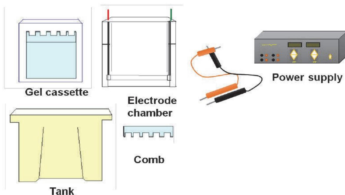
**Fig.34. SDS-PAGE Instrument**
