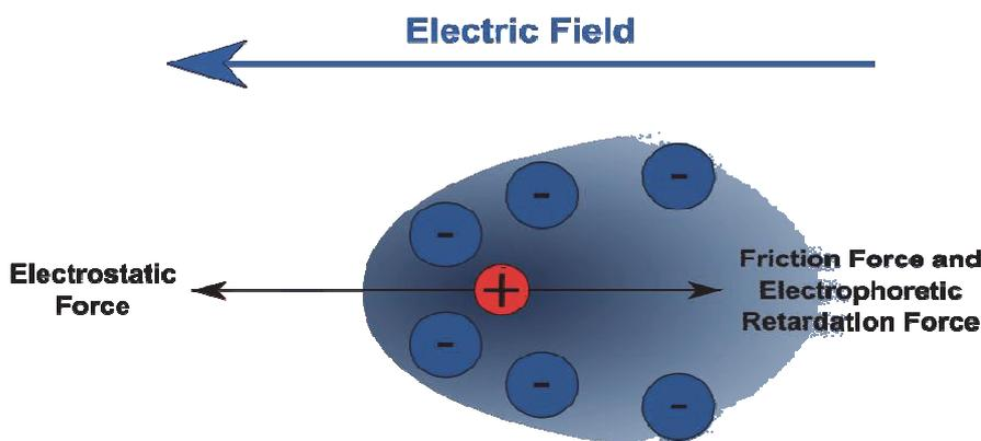
**Fig. 32. Movement of charged particles in an electric field**
