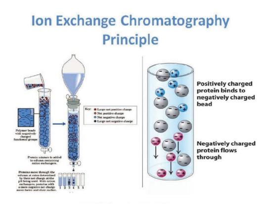
Fig.37. Ion Exchange Chromatography
