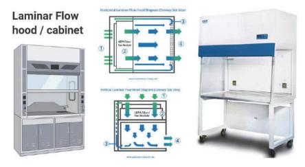
Fig.13. Laminar air flow cabinet
