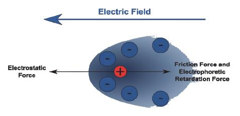
Fig. 32. Movement of charged particles in an electric field
