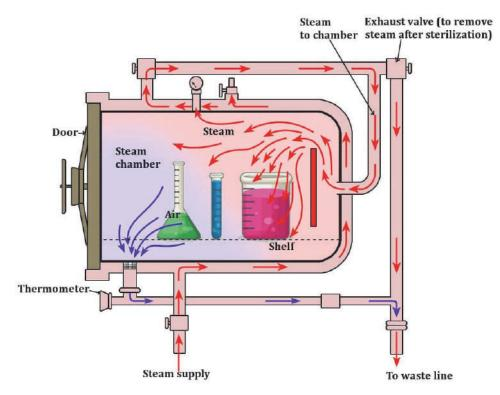
**Fig.24.1.** Principle of Autoclave
