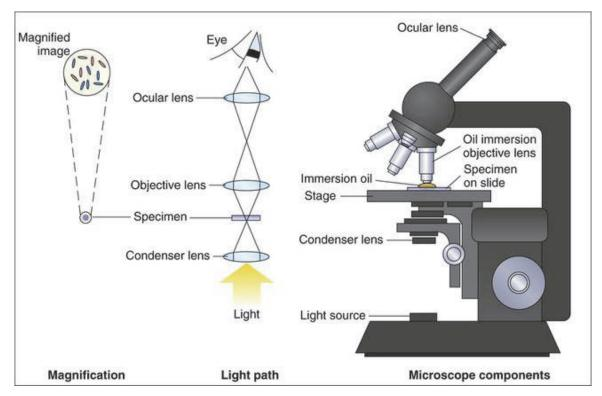
Fig.18.1. Working Principle of a Microscope
