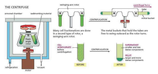
Fig.26.1. Rotors and Centrifugation
